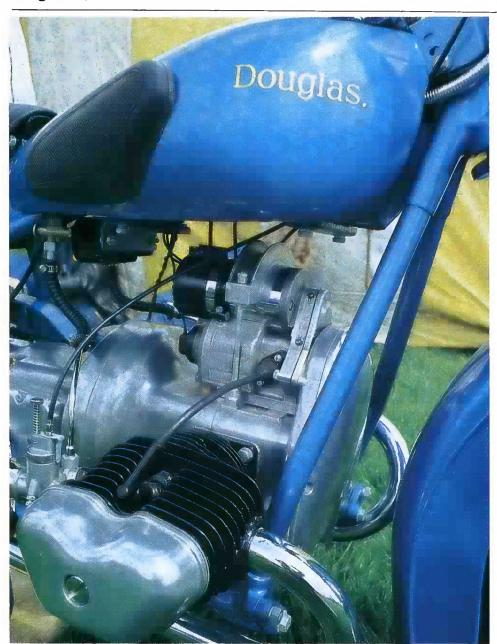
Left: an unusual mounting position for a Lucas Magdyno, atop the crankcase of a flat-twin Douglas Mk V of 1950 vintage. The enclosed drive to the unit can be seen between the front down tubes of the frame
